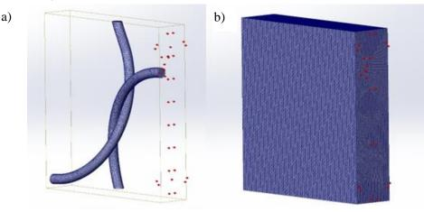
Fig. 2. Mesh in yarn (a) and mesh in unit cell (b)
